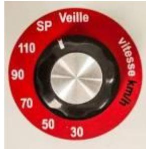
To simplify installation and avoid any computer setup, Evolis radar sign provides pre-set parameters with related to different types of speed limits in force (limited to 30 km / h areas, 50 km / h.). When installing or changing location, just turn the dial to select the correct settings corresponding to speed limit.
